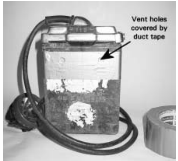
Oldham battery ready for use with vent holes covered by waterproof duct tape IY
